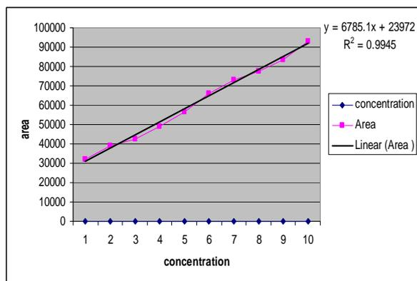
**Fig. 2.** Standard graph of different conc. of pure paracetamol (PCT)
