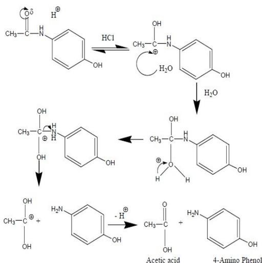
**Fig. 6.** Degradation pathway of PCT in 0.1 N HCl
