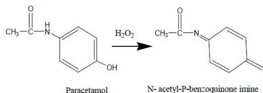
**Fig. 7.** Degradation pathway of PCT in 0.1 N H<sub>2</sub>O<sub>2</sub>
