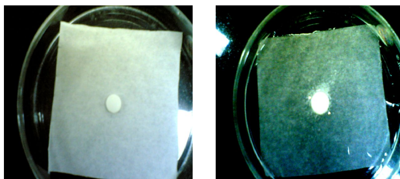
Fig. 1. Wetting time of granisetron hydrochloride ODT
